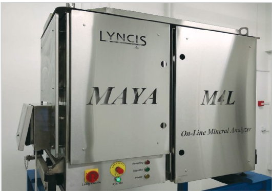
LIBS Spectrometer during Factory Acceptance Test.
